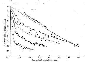
For small pupils (2 mm in diameter) and high spatial frequencies (approaching 50-60 cycles per degree), the human eye is diffraction limited. In other words, no matter how good the optics are, there is a physical limit to the detail that can be resolved--around 60 cycles/degree, the contrast of a 100% contrast grating drops to zero at the retina.
