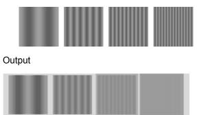
If the input image intensity is  $I(x) = a_f^{in} \cos[2 \pi (f x)] + b$ , contrast is defined as  $a_f/b$ . The modulation transfer function (ordinate in figure from Campbell and Green, below) of an optical system is the ratio of the output amplitude to the input:  $a_f^{out}/a_f^{in}$
